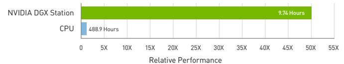
Workload: ResNet-50, 90 epochs to solution | CPU: dual Xeon Platinum 8180, BS=256 | GPU: 4X Tesla V100 32GB, BS=512
